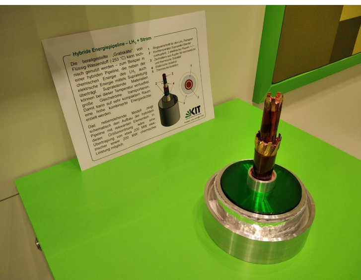
Model of a cable for hybrid pipelines. Photo: Mira Wehr, ITEP/KIT
